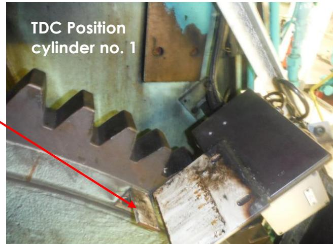
2.3 Install the bracket for TDC pickup.
